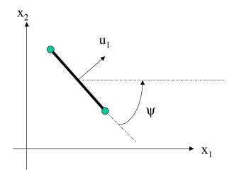
Basically,  $\psi$  is the yaw angle of the vehicle, and  $x_1$  and  $x_2$  are the Cartesian locations of the wheels.  $u_1$  is the velocity of the front wheels, in the direction that they are pointing, and  $u_2$  is the steering velocity.
